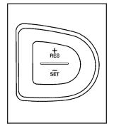
If your vehicle has cruise control, the buttons for the cruise control are located on the steering wheel.
